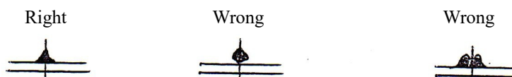
Figure 5. In the middle, the wire has been tinned, but not the soldering point on the card, the opposite case shown to the right. Left, both parts are shown correctly tinned and electrically connected.
